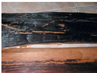
Waterproof inside layer of 2 banana fiber pieces
